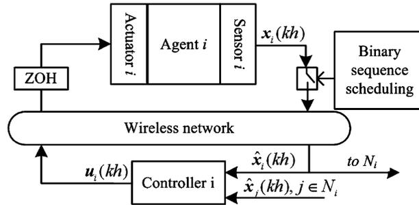
Figure 4 The structure of the agent node
