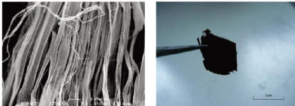
Figure 4. Carbon nanotube array photos (Left: SEM photo; Right: Suspended carbon nanotube array formed by cutting)
