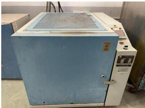
Fig. 1 Box-type resistance furnace
