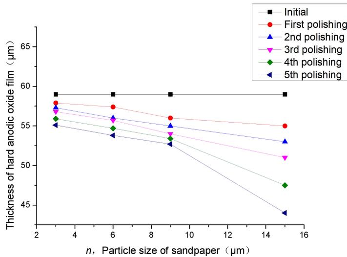
Fig. 13 Comparison of thickness of hard anodic oxide film under different particle sizes of sandpaper
