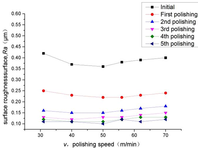
Fig. 8 Comparison of roughness of hard anodized film under different polishing speeds
