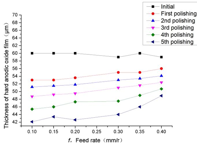
Fig. 11 Comparison of the thickness of hard anodized film under different feed rate
