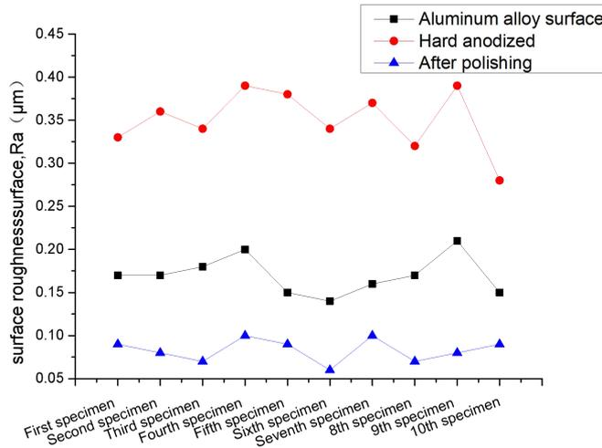
Fig. 2 Comparison of roughness of hard anodized film before and after polishing
