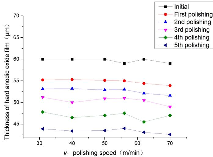
Fig. 9 Comparison of thickness of hard anodic oxide film under different polishing speeds
