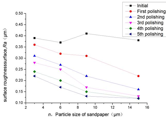
Fig. 12 Comparison of roughness of hard anodized film under different particle sizes of sandpaper
