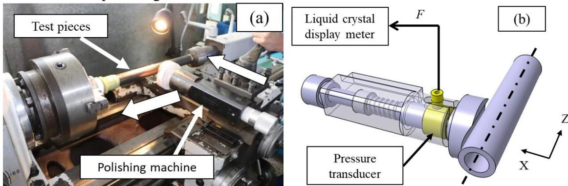
Fig. 1 Schematic diagram of the polishing experimental system and polishing force measurement system: (a) Polishing experimental system (b) Polishing force measurement system
