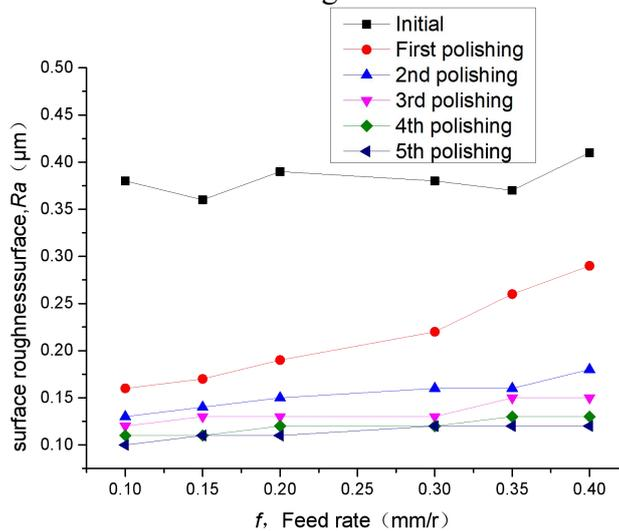
Fig. 10 Comparison of roughness of hard anodized film under different feed rates
