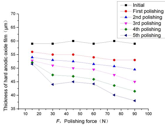
Fig. 7 Comparison of thickness of hard anodic oxide film under different polishing forces
