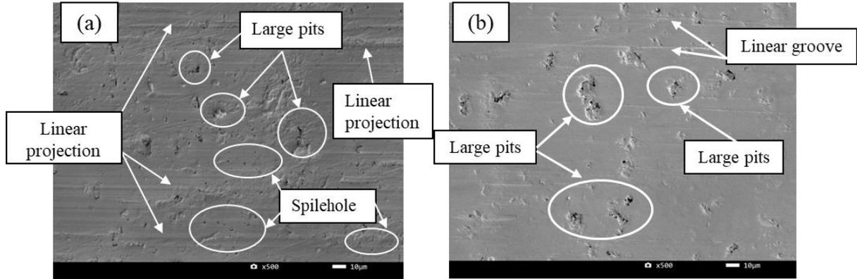
Fig. 5 Comparison of hard anodized film before and after polishing (500x): (a) Before polishing (roughness Ra 0.366) (b) After polishing (roughness Ra 0.082)
