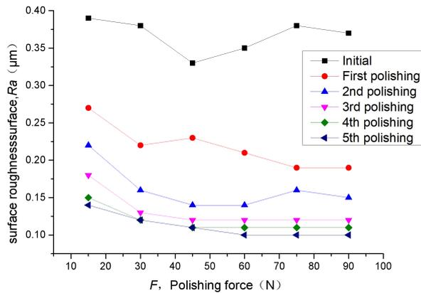
Fig. 6 Comparison of roughness of hard anodized film under different polishing forces
