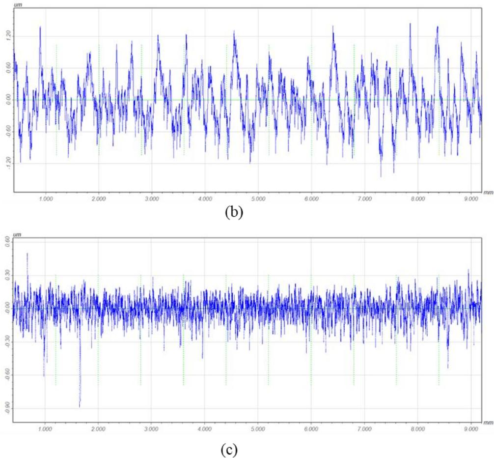
Fig. 4 Roughness measurement curve: (a) Aluminum alloy surface (roughness Ra0.140) (b) Hard anodized (roughness Ra0.366) (c) After polishing (roughness Ra0.082)
