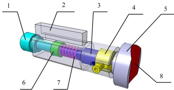
Fig. 2 Joint diagram of polishing device :1-Plug, 2-Base, 3-Arbor, 4-Pressure sensor, 5-Polishing head, 6-Positioning sleeve, 7-Spring, 8-Abrasive paper
