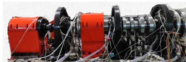
Figure5. Twin rotor test rig with mid turbine frame structure
