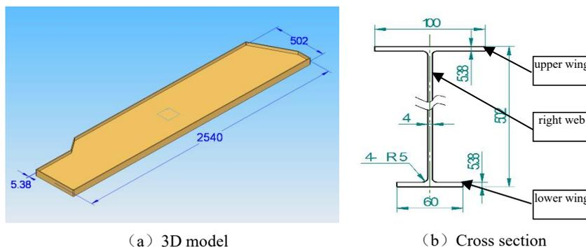
Figure 1. Three-dimensional model and cross-section diagram of I-shaped closed beam
