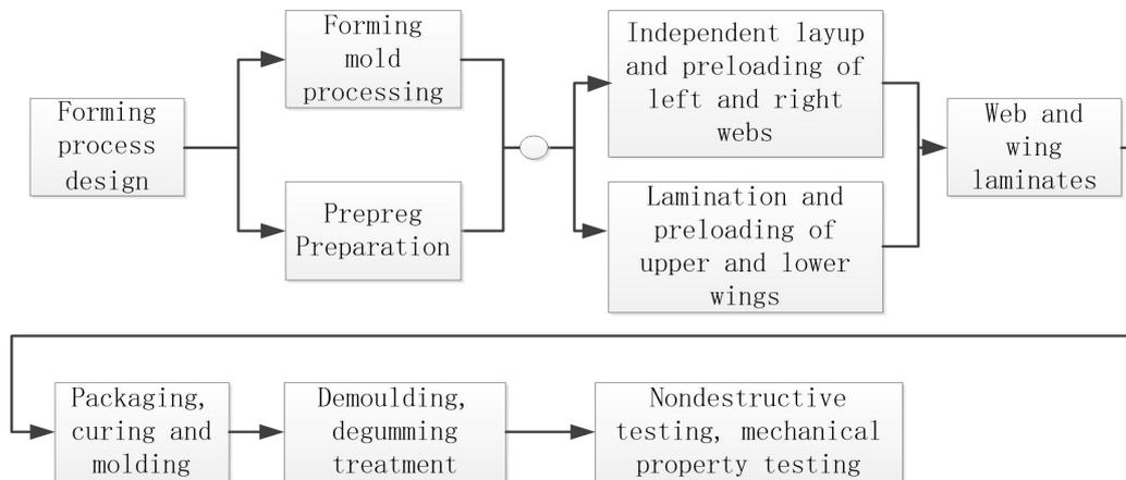
Figure 2. Process flow chart of closed beam
