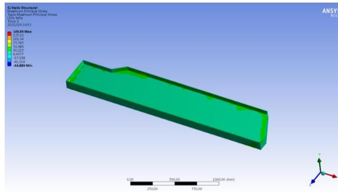
Figure 6. Curing stress cloud diagram of closed beam products
