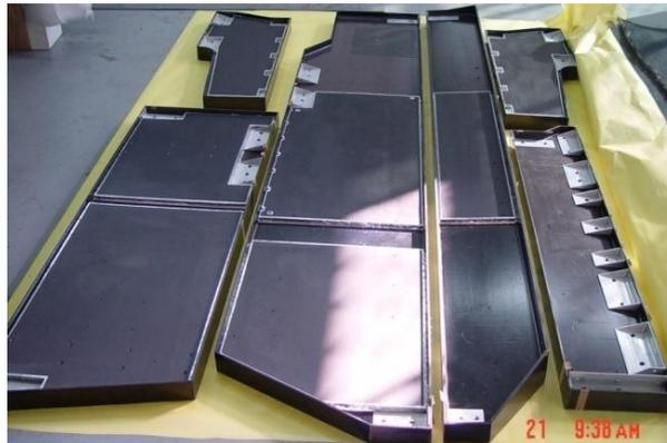
Figure 8. Many pieces of large-size I-shaped composite material closed beams
