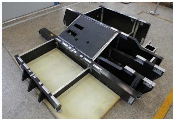
Figure 9. The physical assembly of the large-size I-shaped composite material closed beam assembly structure
