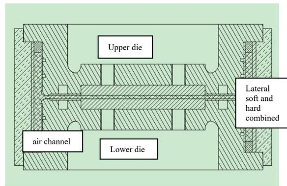
Figure 3. Schematic diagram of the structure of the closed beam curing forming mold
