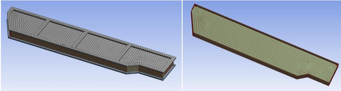
Figure 4. The closed beam product and the finite element model of the solidified forming mold
