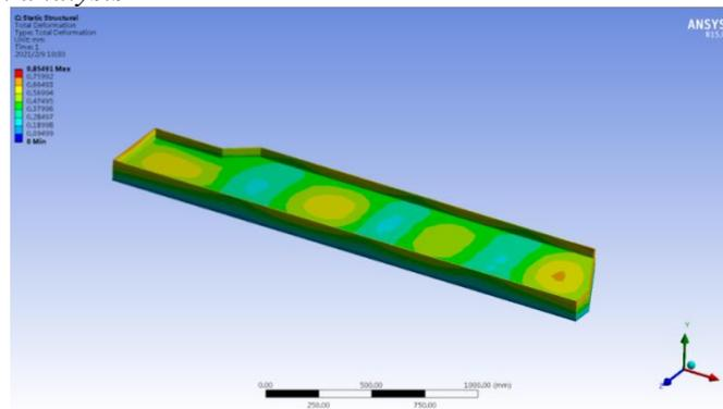
Figure 7. Curing deformation cloud diagram of closed beam products
