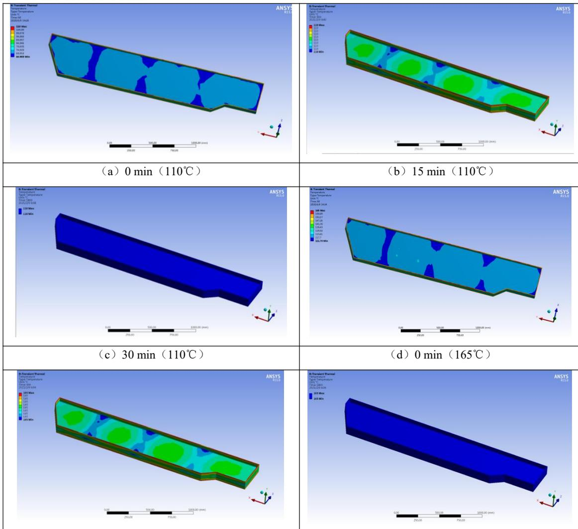
Figure 5. Temperature distribution at the inflection point of the closed beam product on the curing process curve
