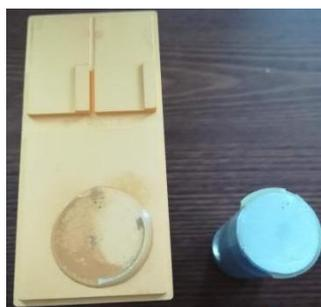
**Figure 2.** Pull off force test of gold coating on the surface of heat sink substrate
