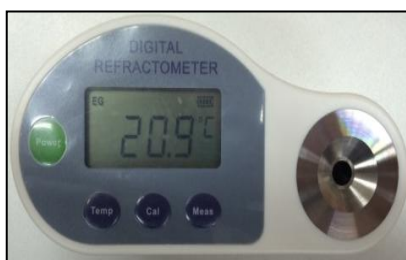
Figure 1: Portable freezing point tester
