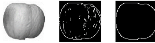
Fig.5 Sobel operator and Canny operator labeling result graph
