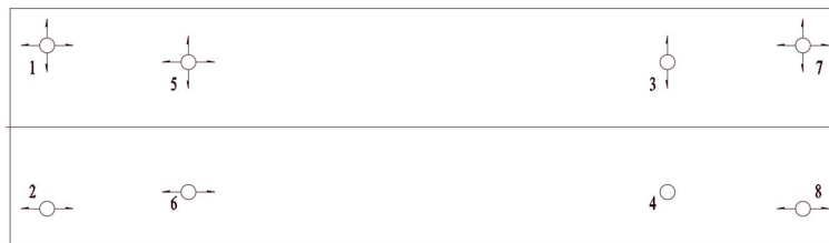
Fig. 2 Arrangement of basin-type rubber bearings
