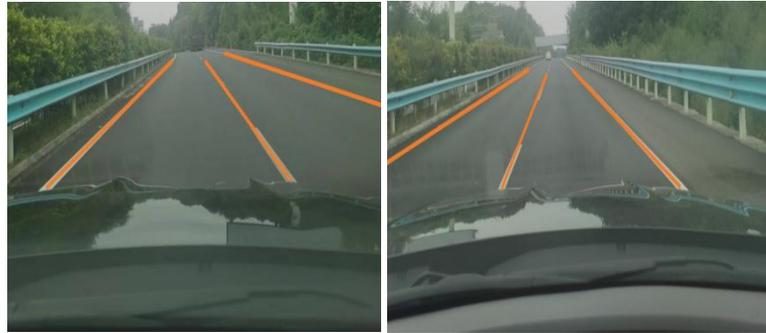
Figure 4. First detection results of lane
