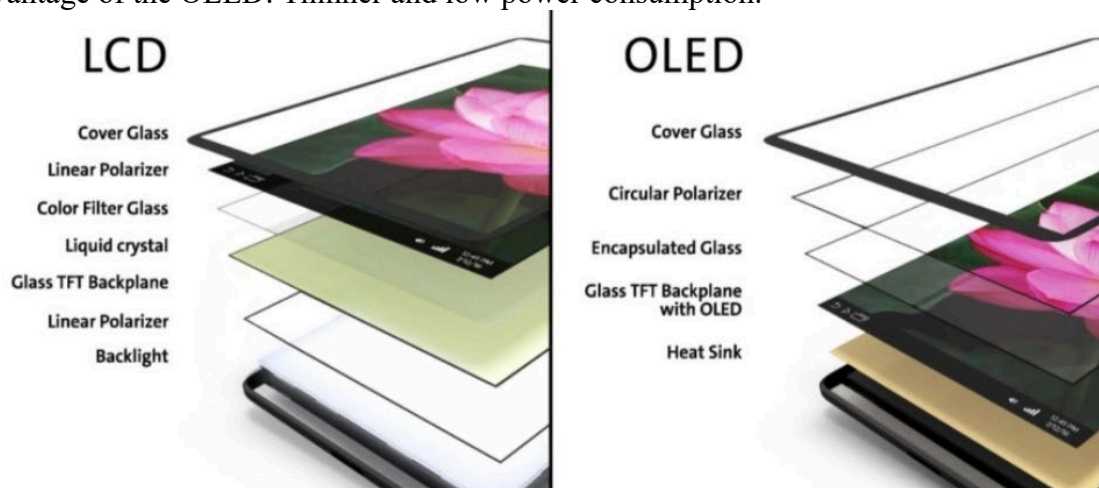
Fig 2 The different structures of OLED and LCD
