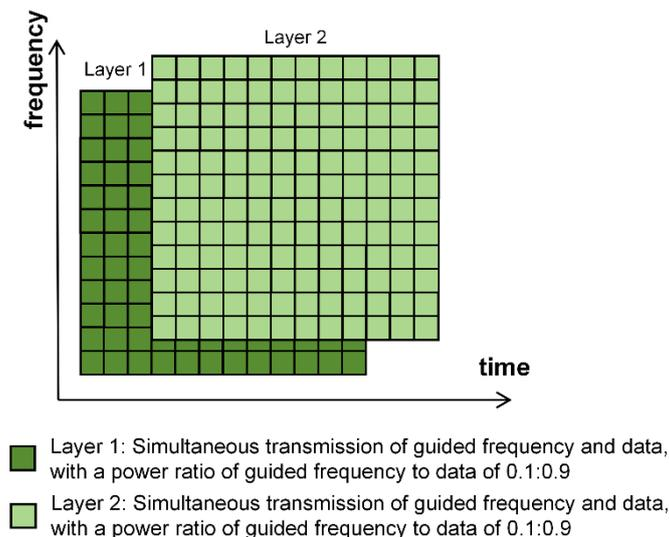
Fig. 5 Overlay configuration of guide frequency and data.
