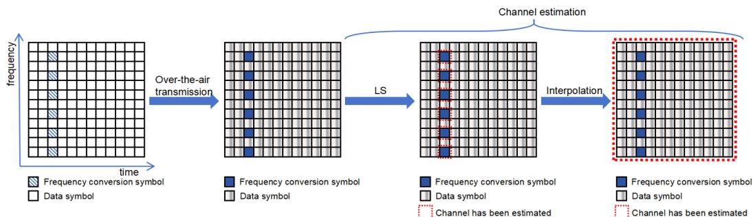
Fig. 1 Quadrature guides in existing communications  $Y = H[X_D; X_P] + N$ .
