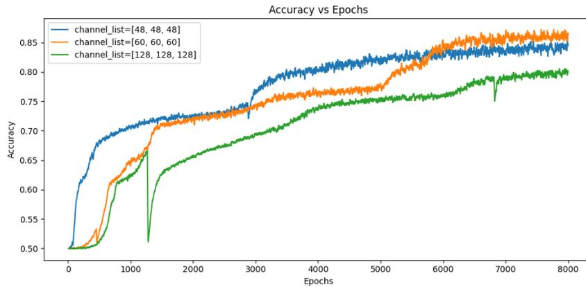
Fig. 6 Receiver data recovery accuracy with different channels
