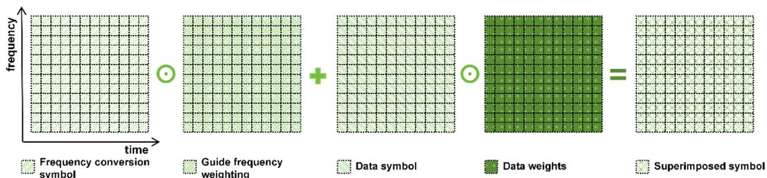
Fig. 3 Non-orthogonal frequency guides with data superposition  $Y = H[XD+XP] + N$
