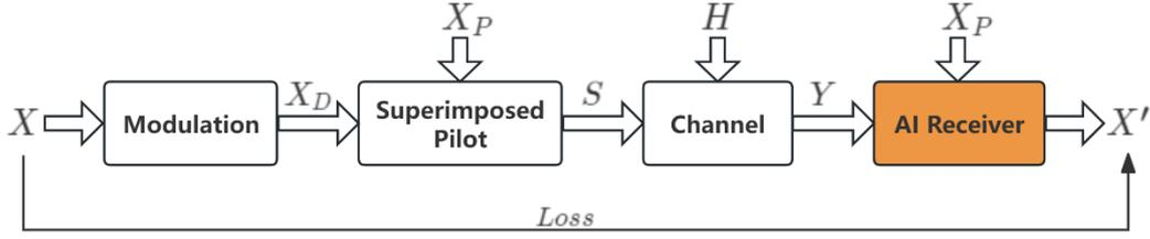
Fig. 2 Transmission process of non-orthogonal guide frequency with data superposition
