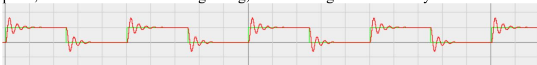
Figure 4: Falstad simulated step response of analog computer.
