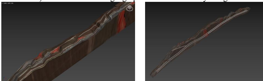
b) Railway topographic and geological model; c) Geological model of railway tunnel
