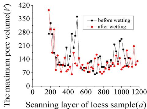
Fig. 6 The maximum pore volume before and after wetting
