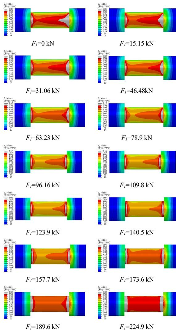
Figure 4. Stress Nephogram of Bolt Surface under Different Initial Preload  $F_1$
