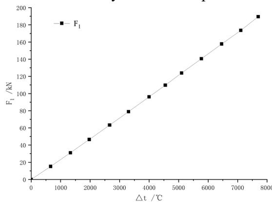
Figure 3. Relationship Between Initial Preload and Temperature Change Rate
