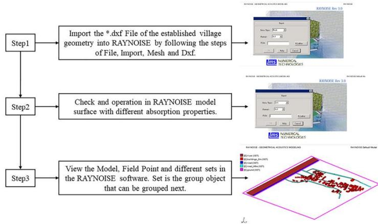
Fig. 2 Steps of importing the geometric model into RAYNOISE software
