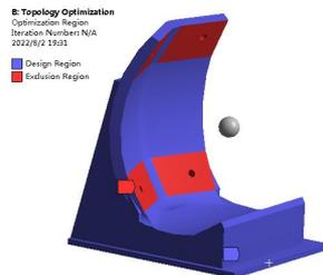
Fig.2 Topology calculation model
