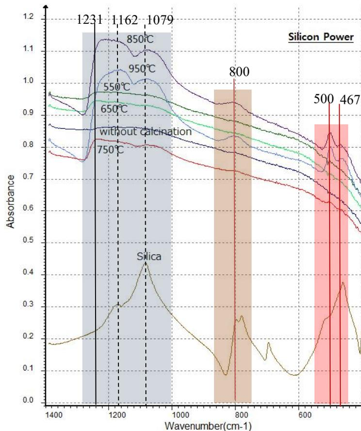
Fig.1 FTIR spectra of silica powder calcined at different temperatures
