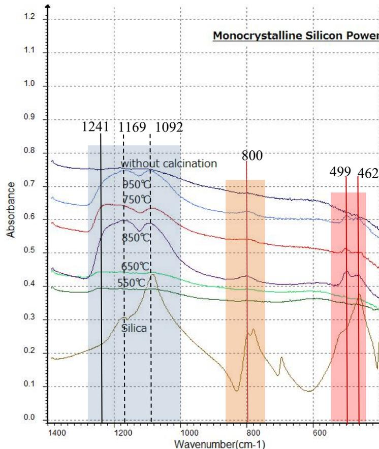
Fig. 2 FTIR spectra of monocrystalline silicon powder calcined at different temperatures
