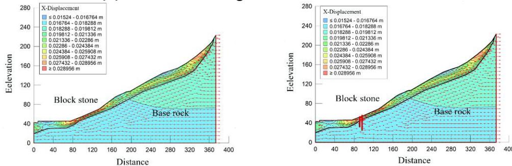
Fig. 4 Displacement map in X direction before and after reinforcement
