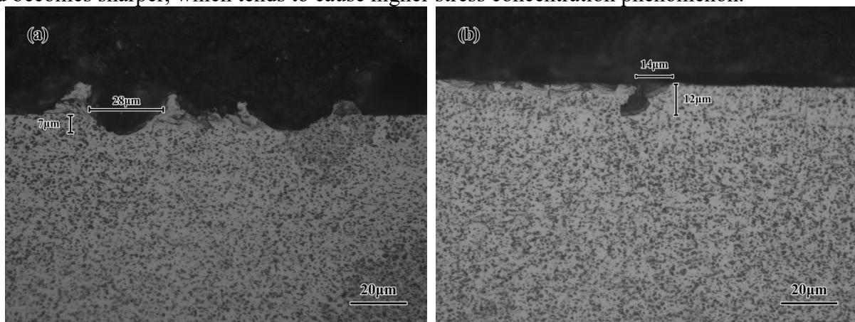
Fig. 2 OM image of the laser marking after : shallow (a) and deep (b)
