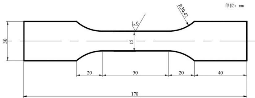
Fig. 1 Schematic diagram of fatigue specimen
