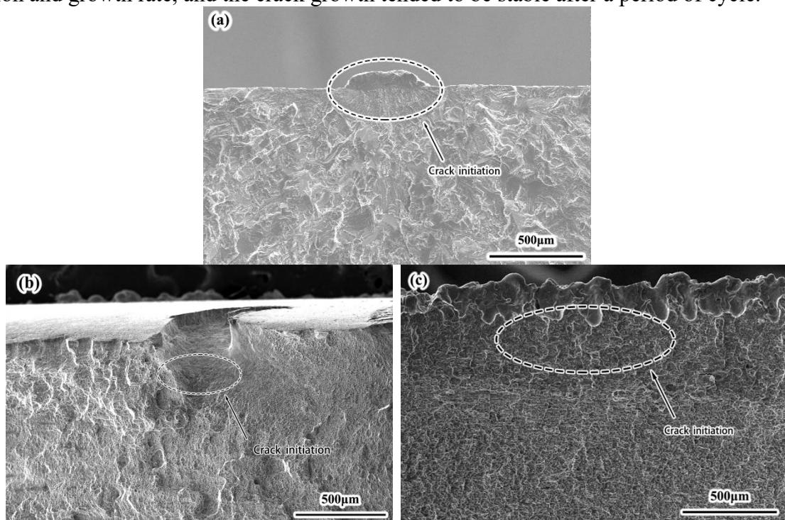
Fig. 3 Fatigue fracture of TA15 titanium alloy after laser marking : unmarked (a)、 shallow (b) and deep (c)
