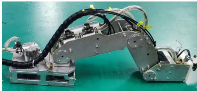
Fig. 7 The assembly of the angle feedback device is complete
