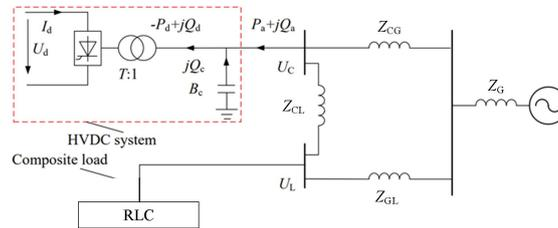
Fig. 1 HVDC equivalent receiving network
