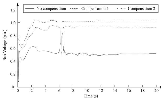
Fig. 5 Voltage changing curves at different compensation positions
