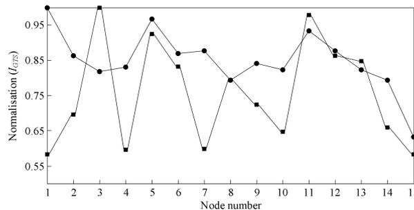
Fig. 4 Normalized nodal voltage reactive power improvement trajectory sensitivity metrics
