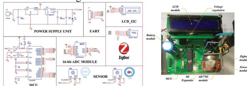
Figure 2: Hardware Diagram of the Lower-Level System
