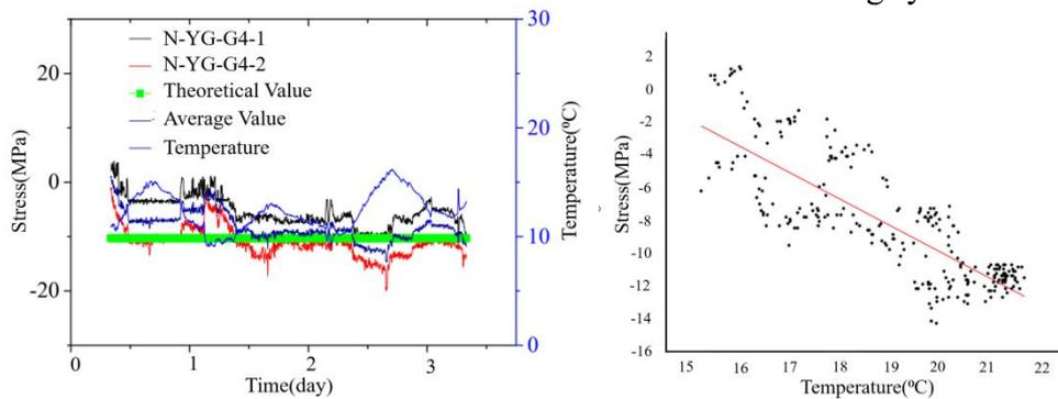
Figure 4: Correlation between Stress and Temperature Figure 5: Graphical Representation of Building Health Monitoring Results
