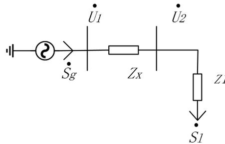
Fig.1 Equivalent line model
