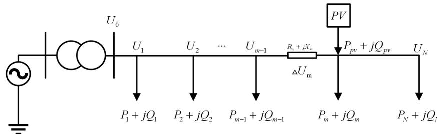
Fig. 2 Typical structure of a low-voltage feeder for a radial distribution network
