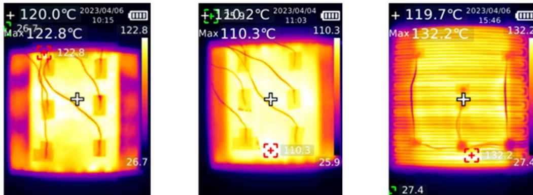
(a)The FGL heater (b)The silicone-encapsulated FGL heater (c)The resistance wire flexible heater
