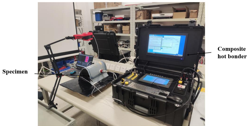
Fig. 7 Schematic diagram of composite single-lap repair experiment on the wing leading edge
