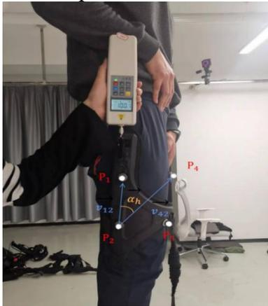
figure 1 The weight bearing gravity and human-machine interaction force of the supporting exoskeleton
