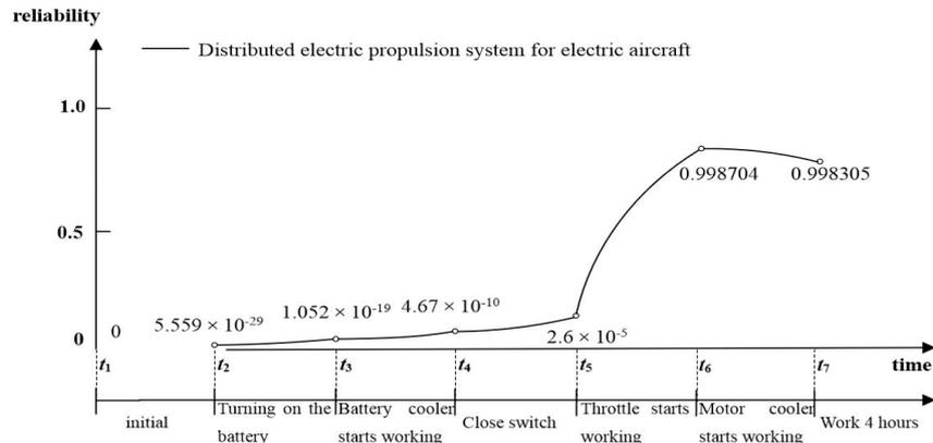
Fig. 7 Reliability Growth Plot for Distributed Electric Propulsion Systems
