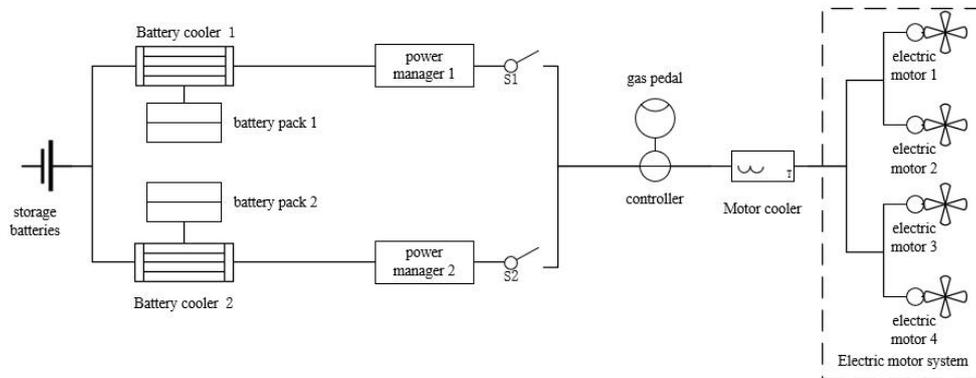
Fig. 1 The Distributed Electric Propulsion System for a certain type of Electric Aircraft
