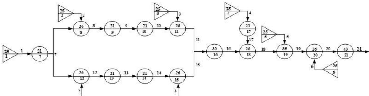
Fig. 6 GO-FLOW Model for Distributed Electric Propulsion Systems in Electric Aircraft
