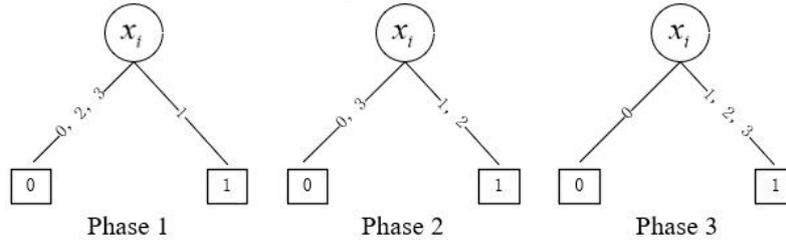
Fig. 3 MDD Structures of Basic Events in a Three-Stage PMS
