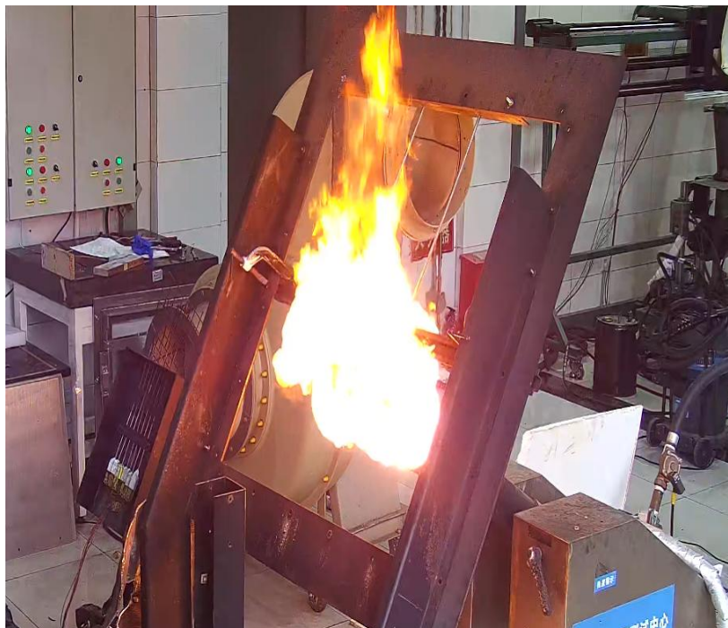
Fig. 4 Emergency locator transmitter burning experiment
