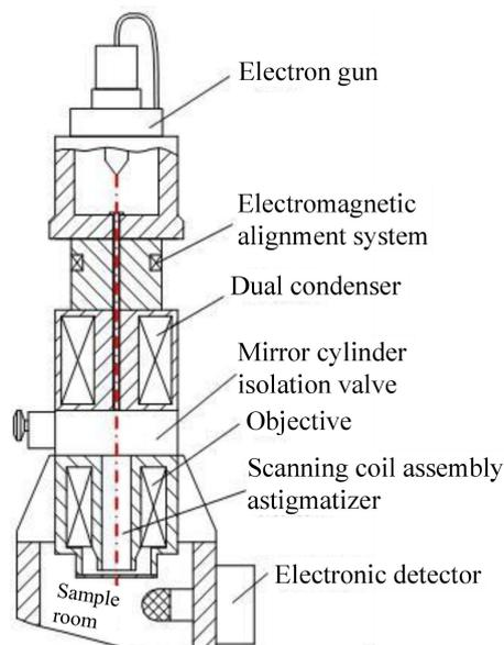
Figure 1. Electron microscope structure
