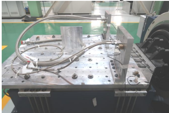
Fig. 3 Installation status of urine collection hose for sinusoidal vibration and random vibration test
