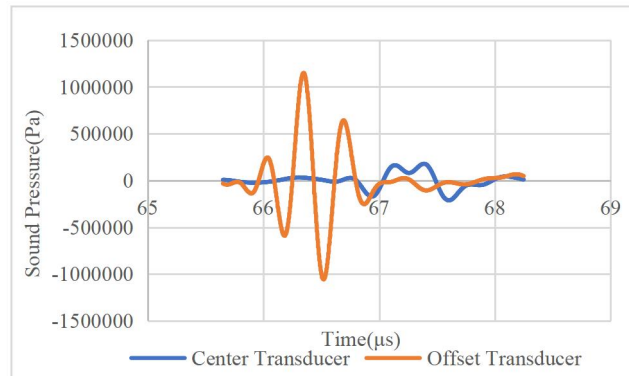
Figure 9 Defect echo waveform under two excitation arrangements
