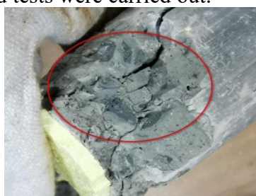
Fig. 8 The failure plane of cement mixed pile
