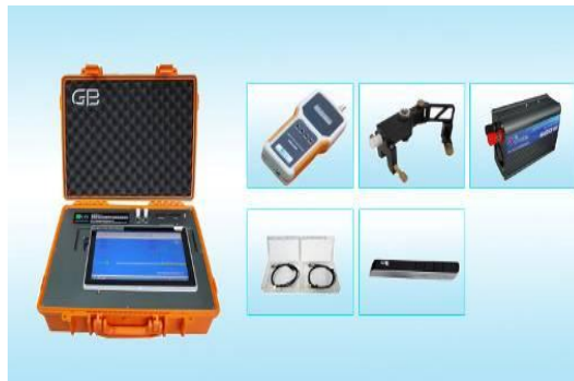
Fig. 6. Steel guardrail column buried impact elastic wave detector
