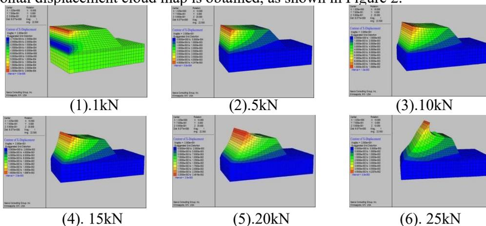
Fig.2 Deformation grid image of horizontal displacement
