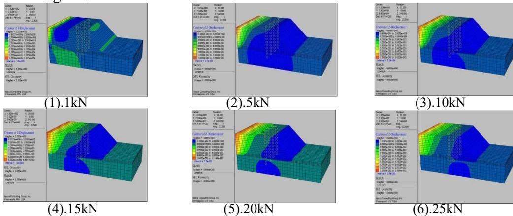
Fig.3 Vertical displacement contour of landslide
