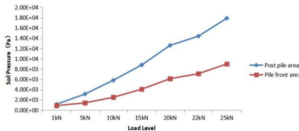
Fig.5 Earth pressure curves in front of and behind piles under different load levels
