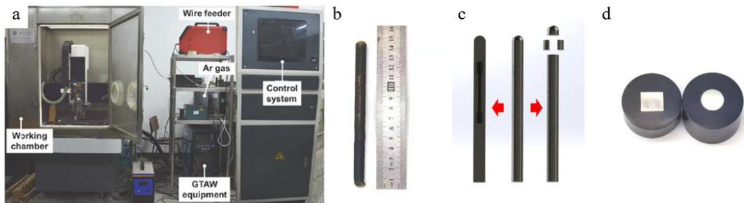
Figure 1. (a) WAAM equipment (b)sample (c)preparation method (the part showing the microstructure is at the top of the sample while the part used to test the mechanical property is at the center); (d)processed sample (including inlaying, grinding, polishing and etching)
