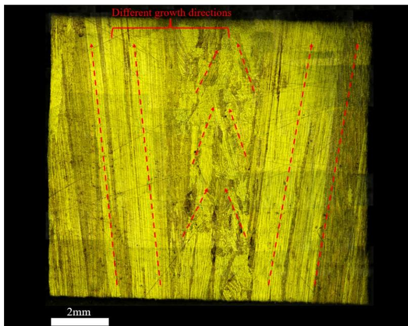
Figure 3. The growth direction of the covering heating columnar crystal
