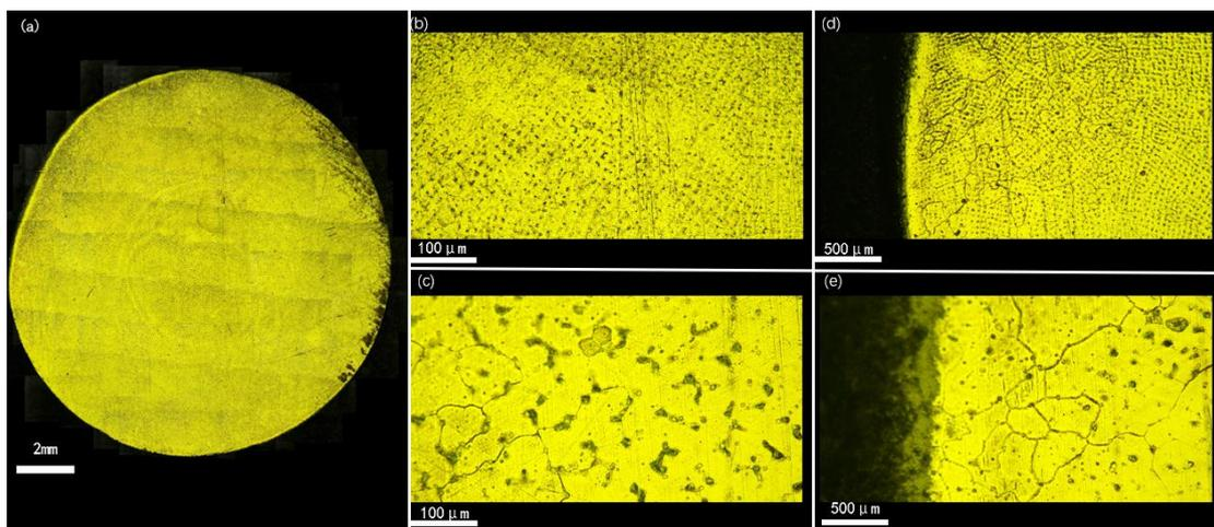
Figure 5. Microstructure at the light microscope (a) the cross section of sample (b) the center part of cross section  $\times 50$  (c) the center part of cross section  $\times 200$  (d) the external part of cross section  $\times 50$  (e) the external part of cross section  $\times 200$
