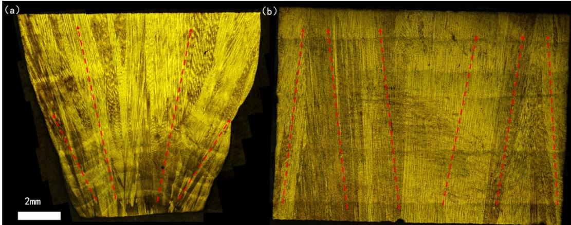
Figure 4. Center heating's growth direction of columnar crystal (a) the metal just grew from the substrate (b) the growth direction of columnar crystal maintaining stable
