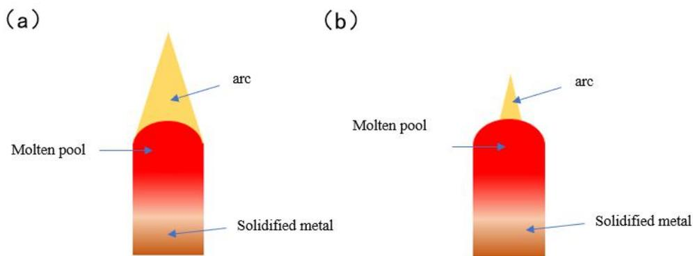
Figure 2. Two heating methods (a) The covering heating that the arc cover the top of the molten pool; (b) The center heating that the arc only cover the center part of molten pool
