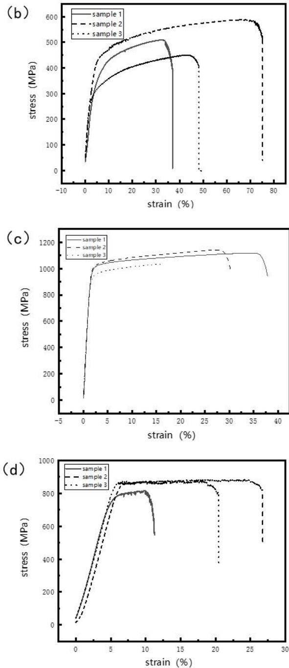
Figure 7. Stress-strain curve (a)the Dos at room temperature (DR);(b) the Dos at 650°C elevated temperature (DE);(c) the HT at room temperature (HR);(d) the HT at 650°C elevated temperature (HE)
