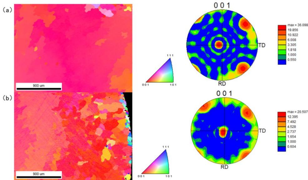
Figure 6. Electron Backscattered Diffraction (a) the center part of cross section; (b) the external part of cross section
