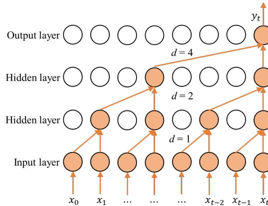
Figure 2 TCN expansion causal convolution structure
