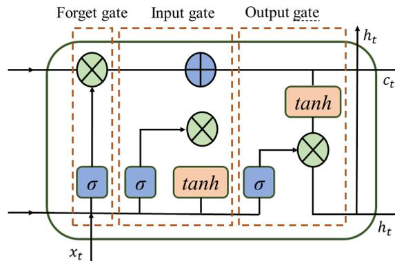
Figure 1 LSTM memory cell structure
