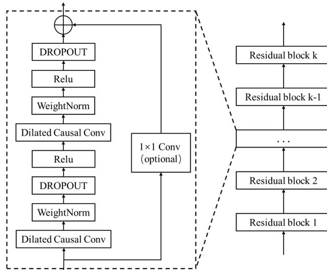
Figure 3 Residual module structure diagram
