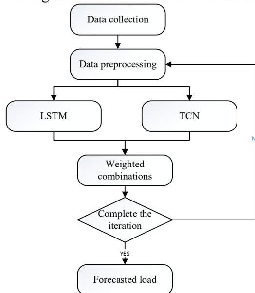
Figure 4 Combined forecasting model flow chart of LSTM and TCN
