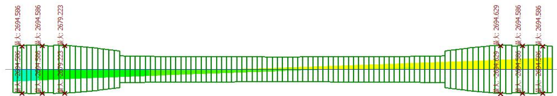
Fig. 10 Envelope diagram of shear bearing capacity of middle beam (unit: \text{kN} )
