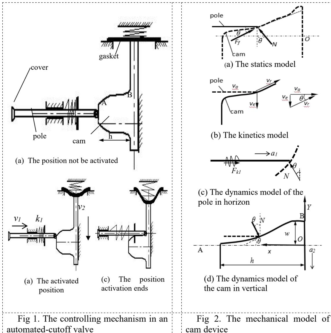
Fig 1. The controlling mechanism in an automated-cutoff valve
