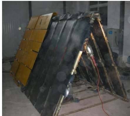
Fig.4. KJ-1 type self-moving emergency rescue support system physical diagram
